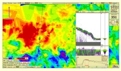
Raw data from the sounder are sent to Olex, so that the system can calculate the seabed topography and hardness. The calculation is done based on the seabed's ability to reflect sound signals, adjusted for factors that can affect the measurements. The system considers parameters like: pulse-length beam-width and transducer type in order to calculate a bottom echo based
