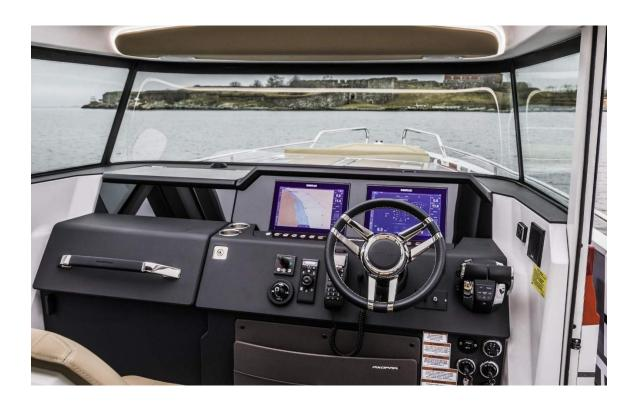
The bridge was produced in partnership with **Simrad-Naviop** and has a single ultra-wide screen displaying all the main monitoring and navigation information, a mix of video sources and clusters of content chosen using the commanders, or two touch screens duplicated by two physical joggers for extra redundancy and safety.
