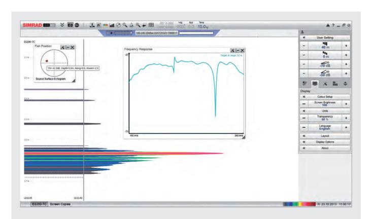
Range resolution and target ID are improved. Echo from a 38,1 mm tungsten sphere is measured, and you can clearly see how the target strength changes with frequency. This frequency response is unique to this particular target, and corresponds well with the theoretical curves. Resolution is excellent, and you can clearly see the knot on the fishing line where the suspended sphere is attached to the line, around 10 cm from the sphere itself.
