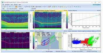
The Echoview license included in an EK80 Portable Entry purchase enables a variety of data processing capabilities, such as target detection, frequency response analysis, and bottom classification.
