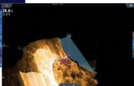
StructureScan 3D's ScanTrack view showing two distinct fish groups of varying species or size holding at different depth contours against this drop off.
