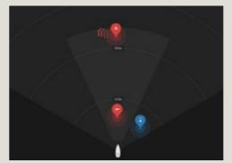
Forward panning. Intelligent alarm alerts of an impending collision risk with objects in the vessel's path.
