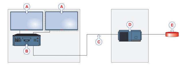
If you want to purchase the Simrad EQ50, you need a computer, a display monitor, a wide-band transceiver and one or more transducers. The EQ50 is a modular system. Each unit is small and easy to install.
