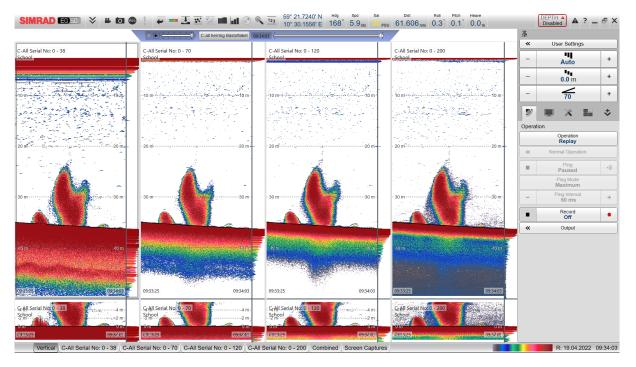
Screen capture: The Simrad EQ50 can handle four different operating frequencies simultaneously. The license includes all these frequencies. This example shows how the EQ50 can present data from a Simrad C-All transducer.
