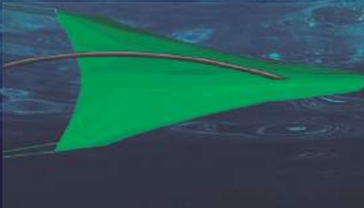
Subsea cable attached to headrope For bottom trawlers with a vertical net opening of <12 meters
