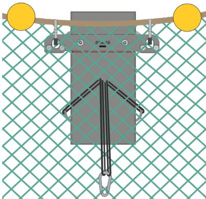
The water flow closer to the net is reduced compared to the flow in the center of the trawl. The built-in ADCP uses the Doppler effect to measure the water speed.
