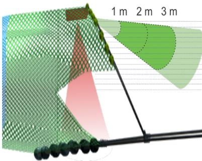
The PX Flow sensor measures the water flow starting 1 meter away from the sensor and in two range cells (cones) of 1 meter each.
